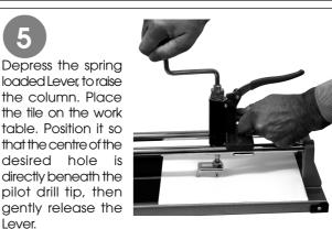
Hold the tile firmly, (or the Steadying Handle, as the operation permits), and begin to turn the Operating Handle **CLOCKWISE**. The pilot drill will begin to drill a pilot hole, and eventually the cutter will come into contact with the tile and a circle will be scored. Continue to turn the handle until the cutter finally breaks through the tile.
