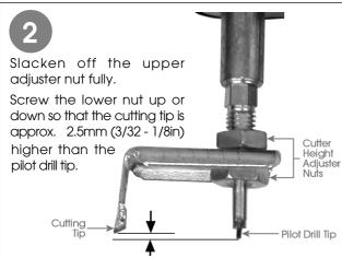
Screw down the upper adjuster nut and lock in place firmly, ensuring the distance from the centre of the pilot drill tip to the outside edge of the cutting tip is set to the desired radius for the hole to be cut.
