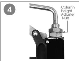
Unlock the Column Height Adjuster Nuts then screw the lower nut clockwise to raise, or anticlockwise to lower, the column, (and hence the cutter), so that the tip of the Cutter is approximately level with, or VERY slightly below, the top surface of the work table.
